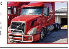
**2002 Volvo VNL 42T,** air ride, flat top, 42" sleeper, Volvo VED-12 425 hp., Eaton FRL 15410C-T2 Auto Top 2, tandem axle, Meritor TR40 - 145 rear axles, 3:73 ratio, diff lock, Volvo 4 bag air ride suspension, duel 100 gal alum fuel tanks, single exhaust, air slide 5th wheel plate, right hand, power windows & mirrors, heated mirrors, A/C, (10) alum wheels, LP 22.5 tires
